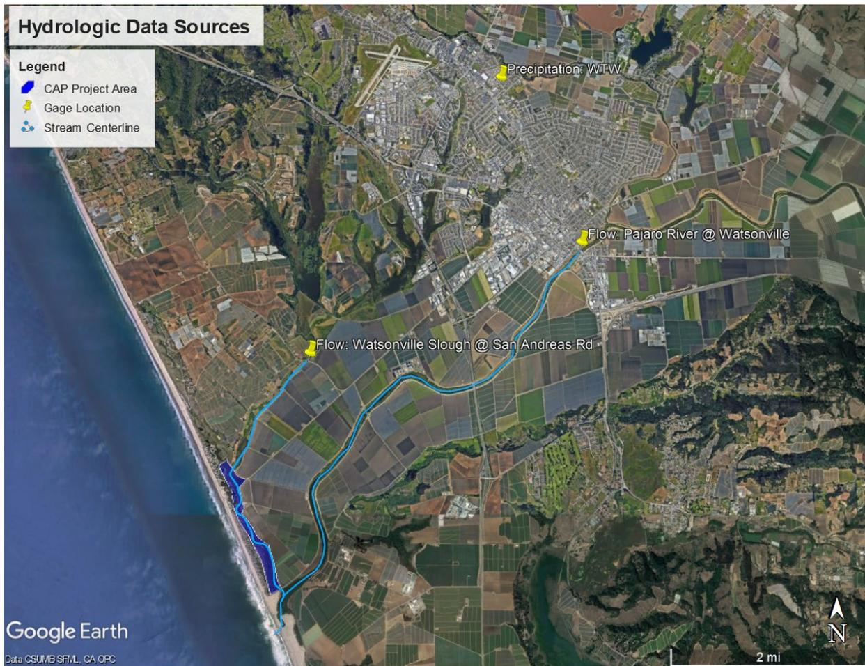
Figure 3: Flow and precipitation gage locations with respect to the project area.
